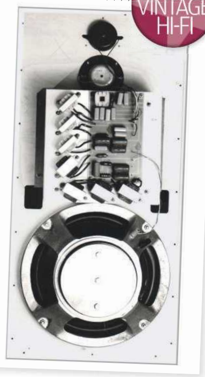
ABOVE: Shot of the rear of the BC III baffle showing drivers and board-mounted crossover
